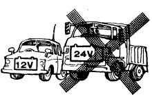
For mobile operation, connect the unit to a 12V car battery (6A). Do not connect it to a 24V battery.
