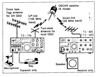
Fig. 16 Example of OSCAR Operation
