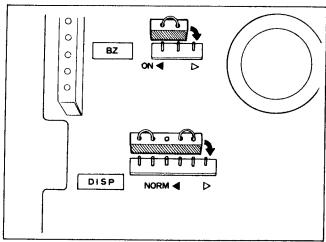
Fig. 3 Select Switches inside Case
